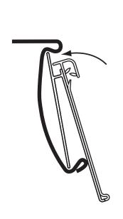
2 Rotate and snap top of back panel into shelf channel.
