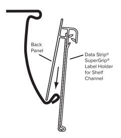
1 Insert bottom of back panel into bottom of shelf channel.
